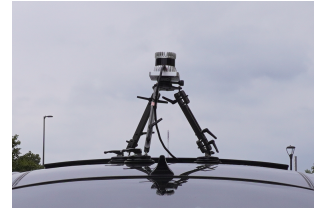
Figure 7: The Ouster OS1-64 LiDAR.
