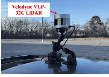
Figure 8: Real-world LiDAR perception testbed.
