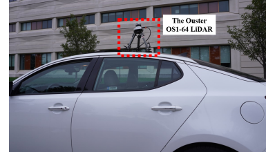
Figure 7: The LiDAR object detection testbed.
