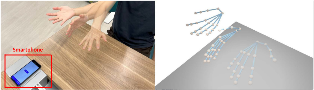
Fig. 1. Illustration of ultrasonic-based 3D hand pose reconstruction.
